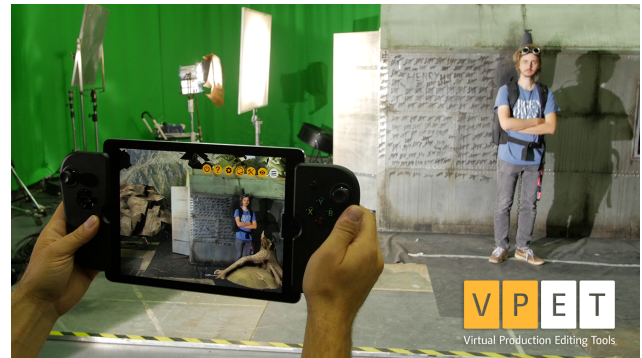
Figure 4: The VPET framework can retrieve its real-time optimised scene from any host application, or ingest USD files containing various LOD’s generated by the system.
